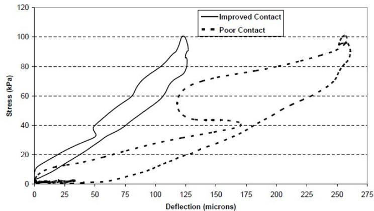
Figure 1. The effect of poor and improved plate-surface contact on the load-deflection trace for a 300mm diameter plate impact test on a well graded crushed rock aggregate.
