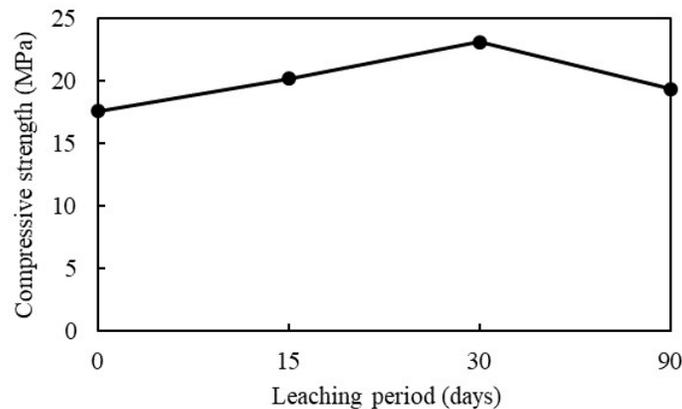
Figure 2. Variations of compressive strength of concrete.
