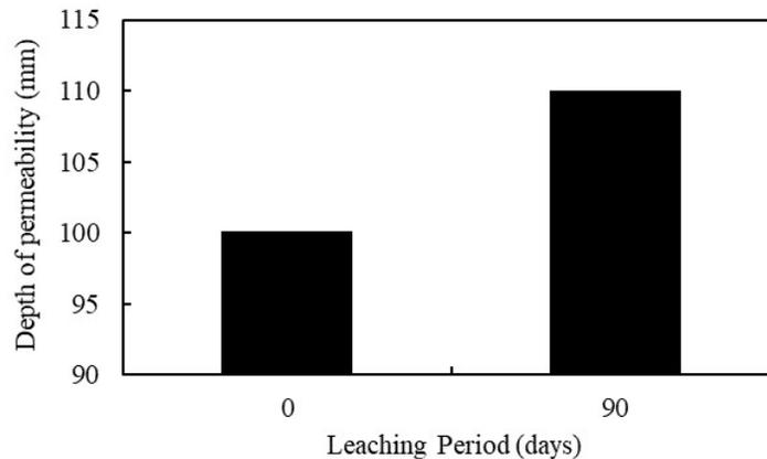
Figure 4. Depth of water permeability of concrete.
