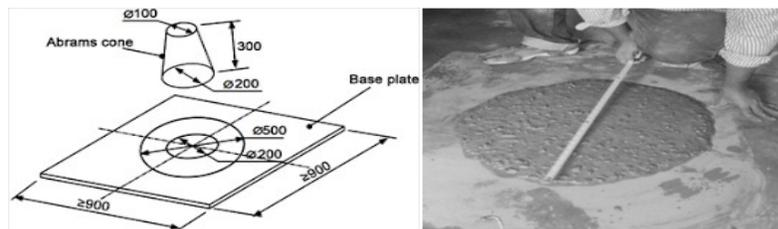
Figure 1. Slump flow test
