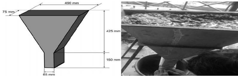
Figure 2. V-funnel test
