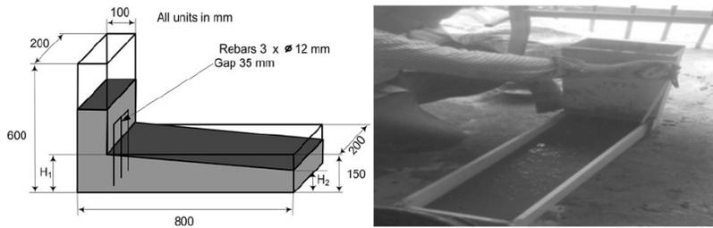
Figure 3. L-box test
