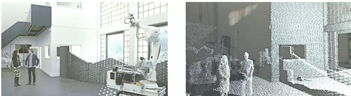
Figure 4. 3D map of the construction site with its 2D laser range-finder by In Situ Fabricator
