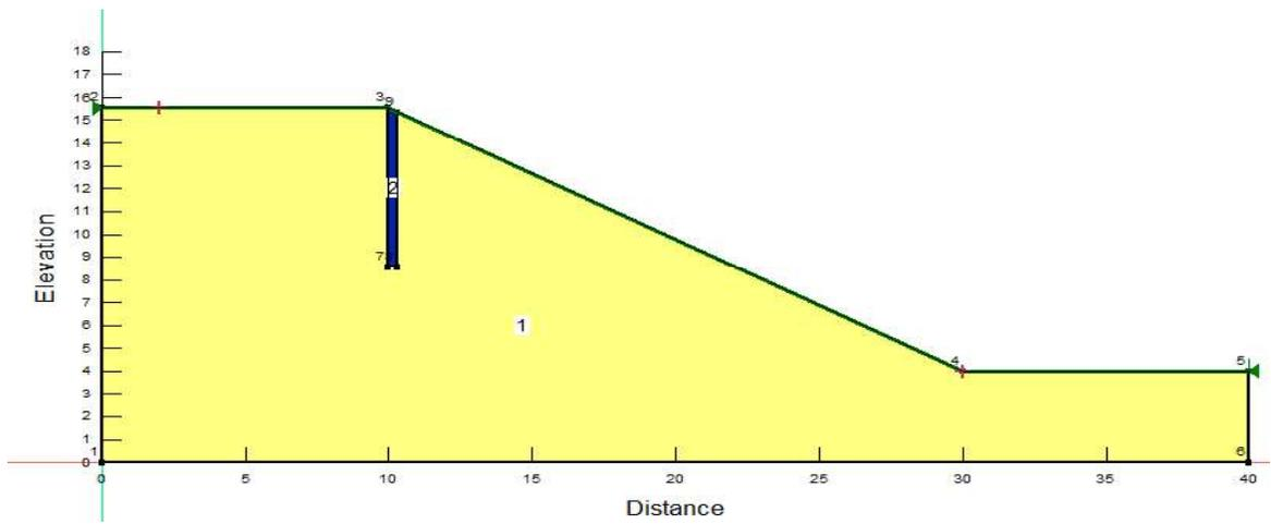
Figure 2: Geometric model of homogeneous earth dam with concrete pile
