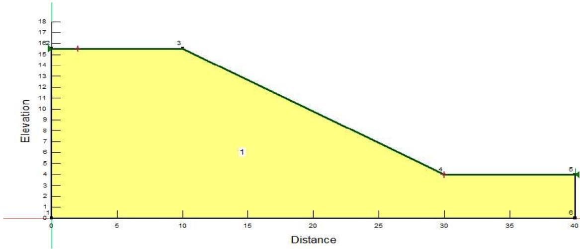
Figure 1: Geometric model of homogeneous earth dam without concrete pile
