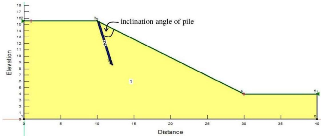
Figure 3: Geometric model of homogeneous earth dam with an inclined concrete pile
