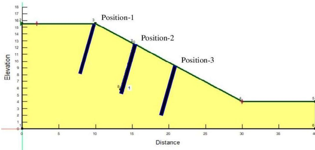
Figure 4: Geometric model of homogeneous earth dam with concrete pile for different positions. Ordinates are: Position 1 (10 m, 15.54 m), Position 2 (15.199 m, 12.54 m), Position 3 (20.398 m, 9.54 m)
