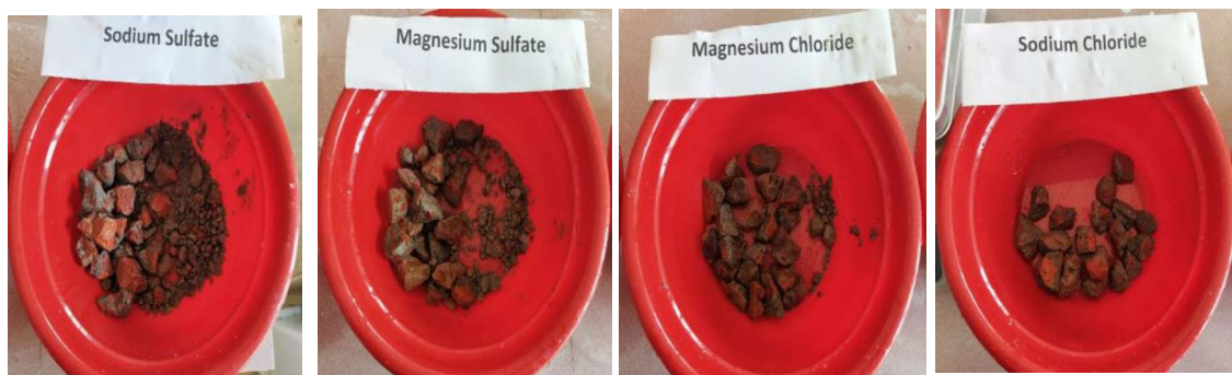
Figure 2. Identification of best performing salt (degradation after 15 days)
