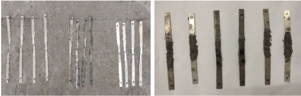
Figure 3. Intersected coupon specimen and CFRP attached coupon specimen
