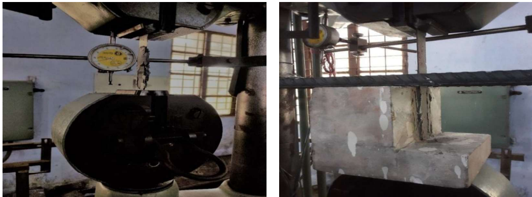
Figure 3. Intersected coupon specimen and CFRP attached coupon specimen
