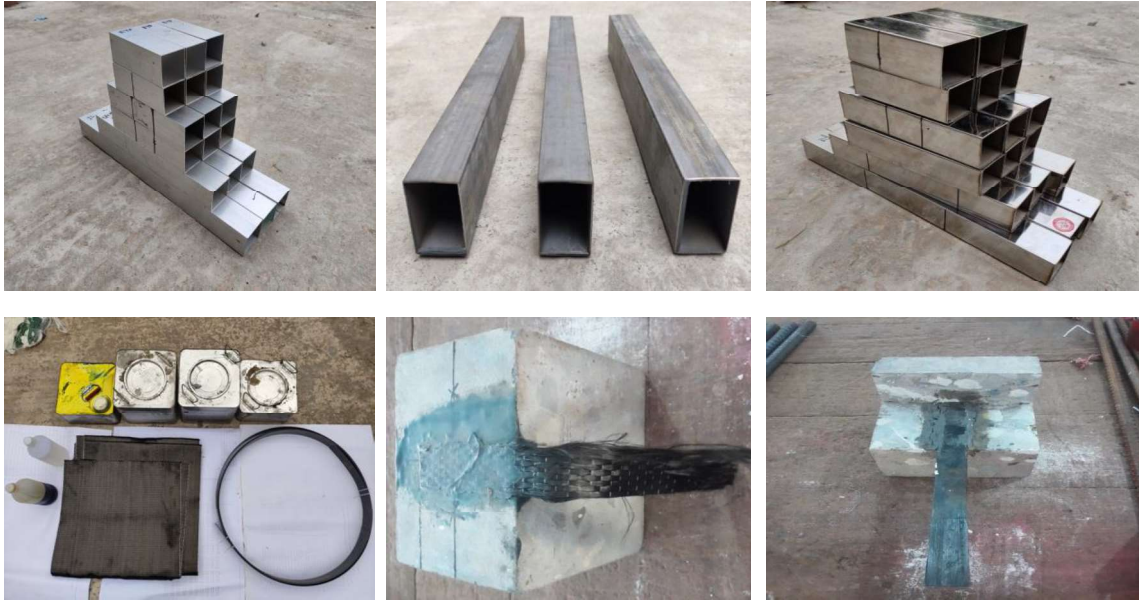
Figure 1. Aluminum, steel, stainless steel, CFRP, adhesive and concrete specimen
