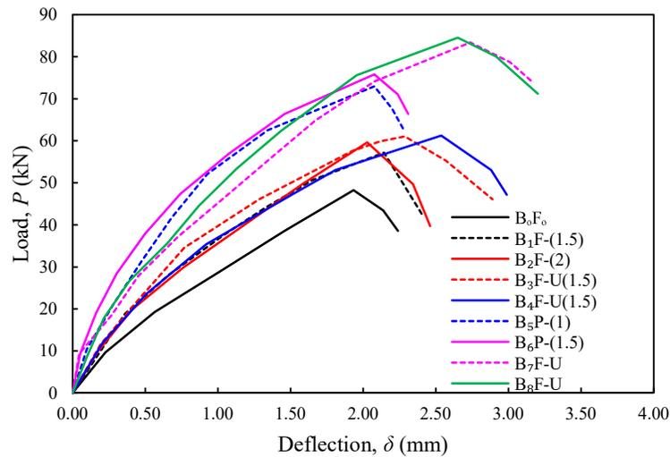
Figure 7. Load-deflection profile of beam specimens
