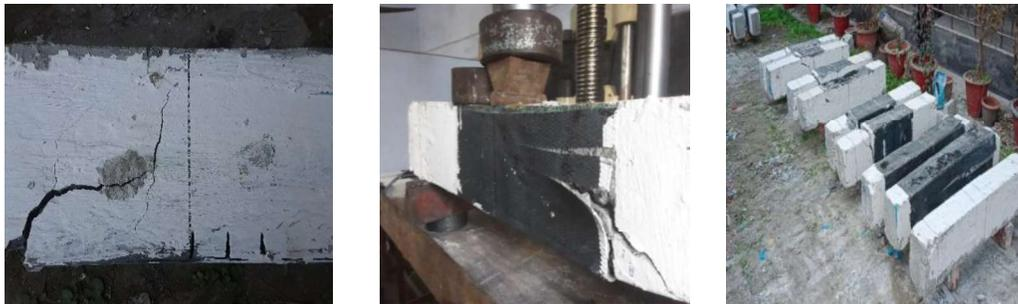
Figure 6. Failure mode of unstrengthen and CFRP strengthen RC beam
