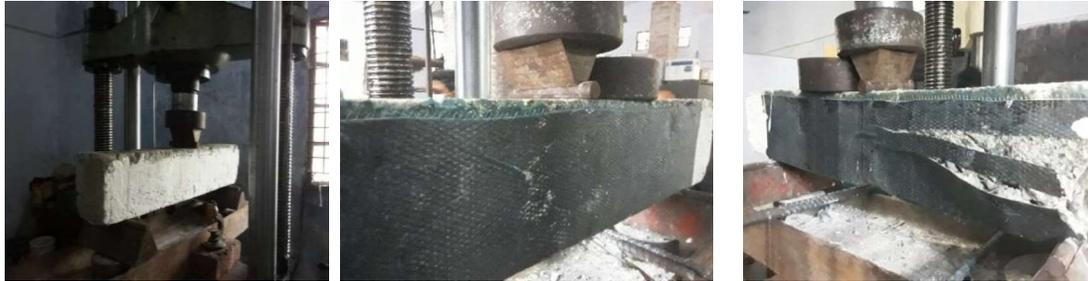
Figure 5. Test setup for 3 point loading of unstrengthen and CFRP strengthen RC beam
