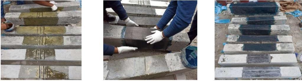
Figure 4. Application of primer-saturant, attaching CFRP sheet, CFRP attached specimen
