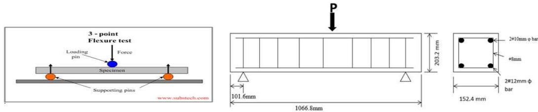
Figure 2. Schematic view of beam dimension in longitudinal and cross section and three points loading
