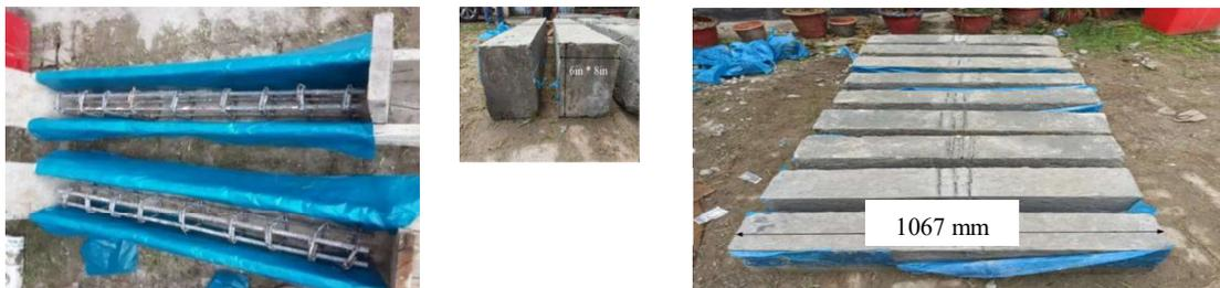
Figurer 3. Reinforcing placed in the mould and pre-cracked RC beam specimen
