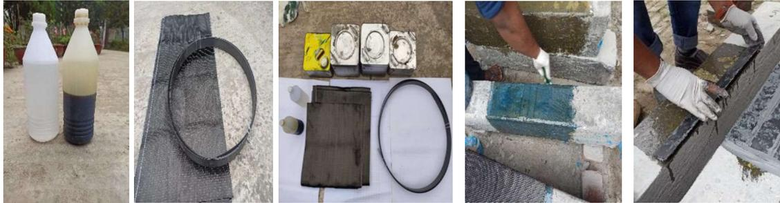
Figure1. Primer & Saturant, CFRP Fabric, CFRP plate, adhesive and concrete beam
