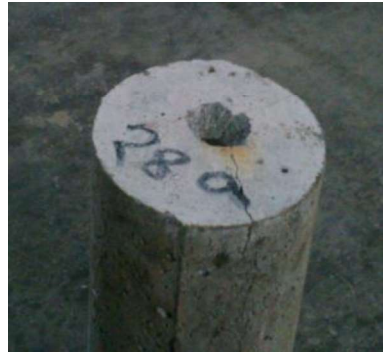
(a) Pullout Failure
