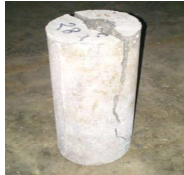
(b) Splitting Failure
