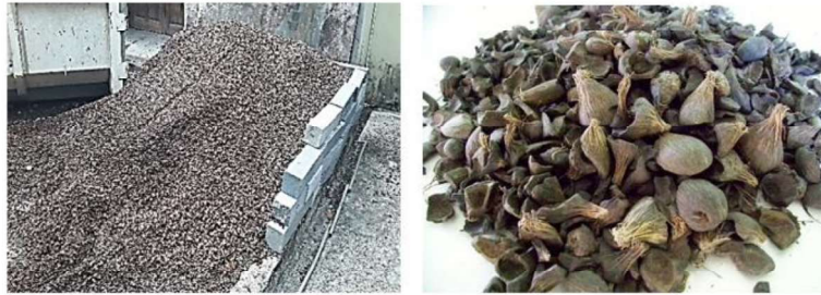
Figure 2. The physical appearance of crushed oil palm shell (OPS).
