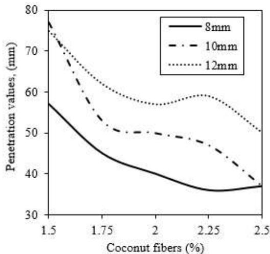
Figure 3: Variations of penetration values with the various percentages and lengths of waste coconut fibers
