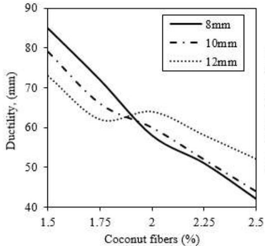
Figure 5: Variations of ductility with the various percentages and lengths of waste coconut fibers
