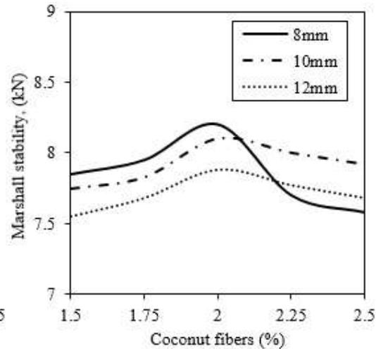
Figure 6: Variations of Marshall Stability with the various percentages and lengths of waste coconut fibers
