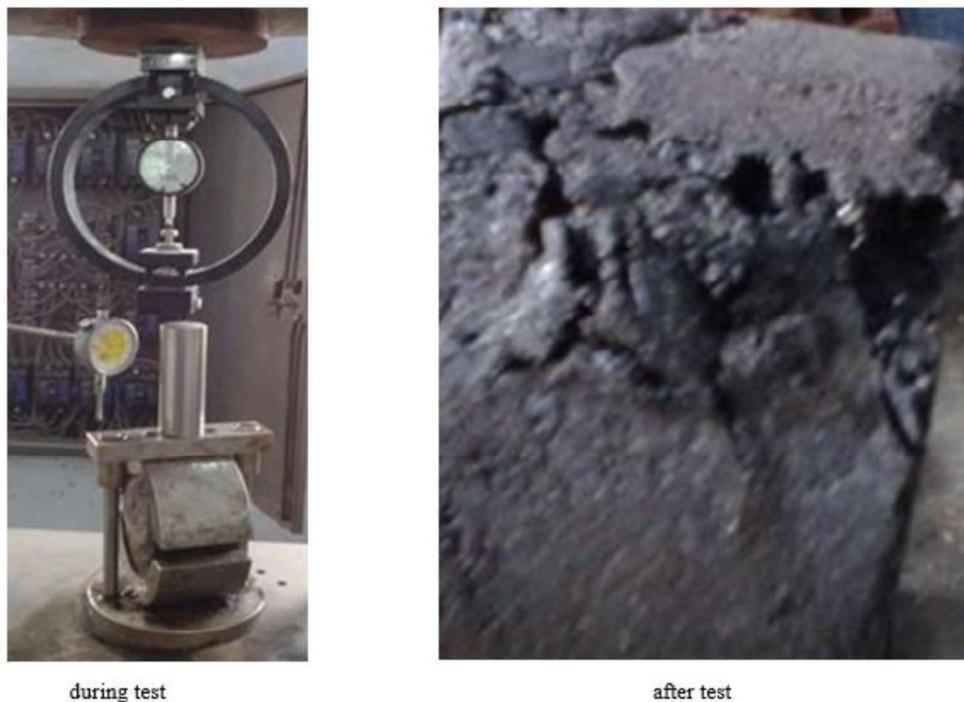
Figure 2: Marshall Stability test procedure and specimen.
