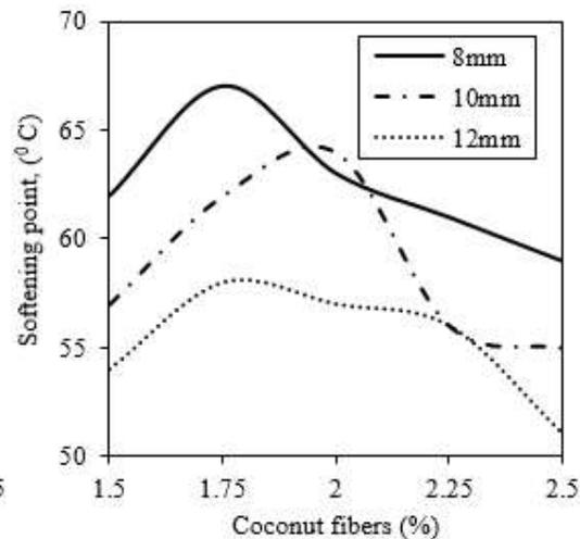
Figure 4: Variations of softening points with the various percentages and lengths of waste coconut fibers
