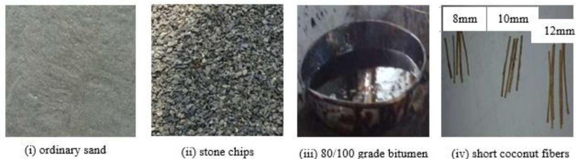
Figure 1: Various types of aggregates, bitumen and additives (coconut fibers)
