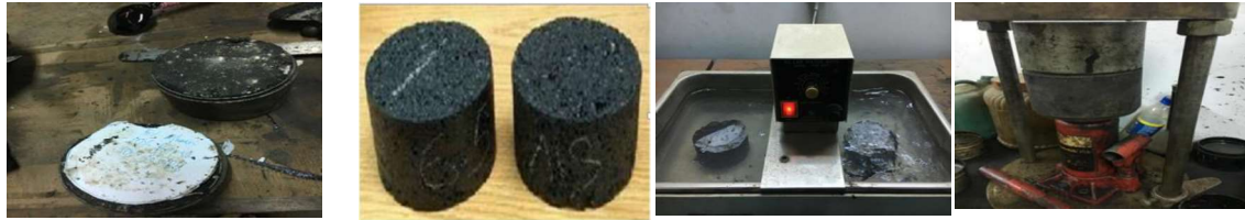
a). Prepared specimens b) Specimens c). Hot water bath d). Marshall Test Figure 2. Steps of Marshall test
