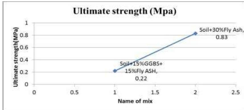
Figure 3: Comparison between Ultimate Strength According to Second Ratio
