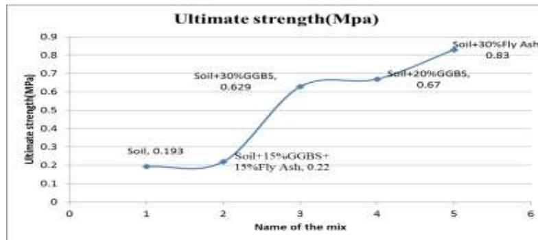
Figure 2: Comparison among Ultimate Strength According to First Ratio
