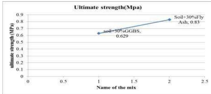
Figure 4: Comparison between Ultimate Strength according to the Third Ratio
