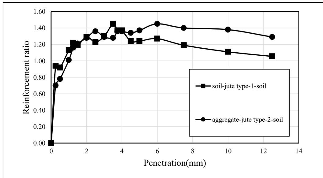
Figure 6. variation of reinforcement ratio with penetration
