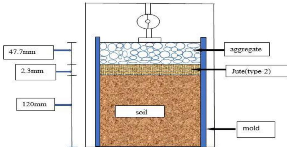
Figure 5. Sample setup for aggregate-jute(type-2)-soil
