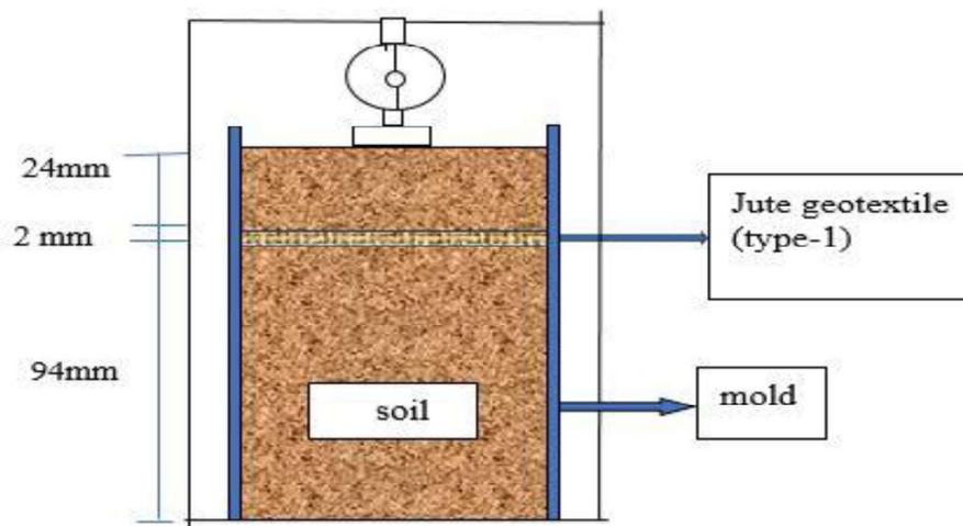
Figure 3. Sample setup for soil-jute(type-1)-soil
