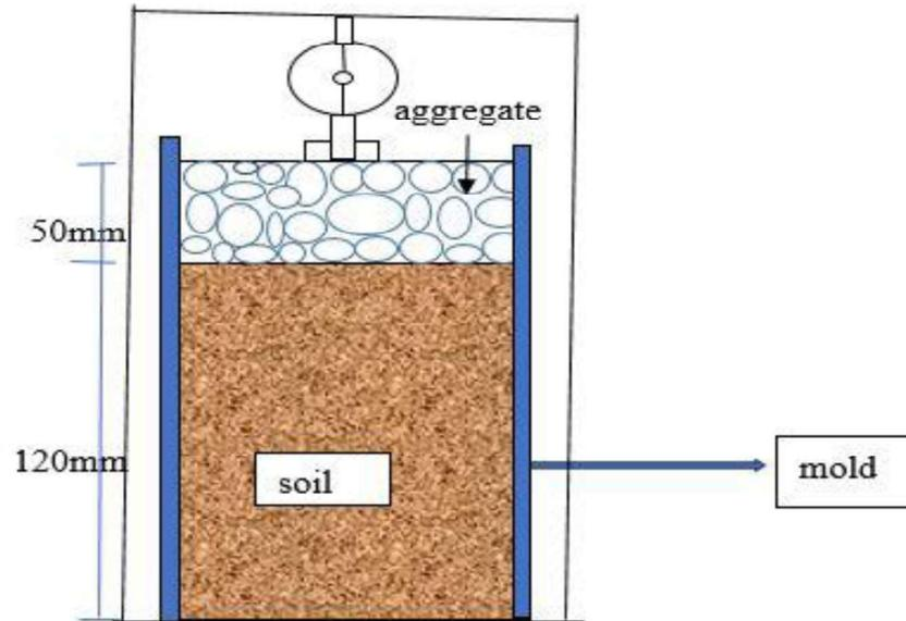
Figure 4. Sample setup for aggregate-soil
