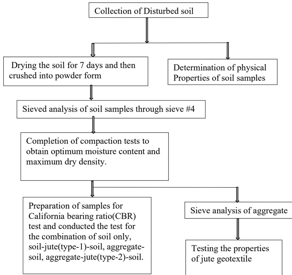
Figure-1. Flow diagram of the task
