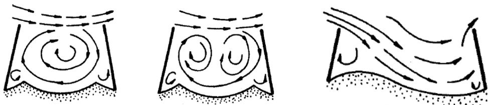
Figure 2: Flow pattern in a spur-field; source: Przedwojski et al. (1995)
