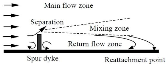
Figure 1: Flow zones due to a spur; source: Zhang and Nakagawa (2008)
