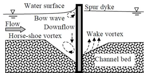
Figure 3: Typical flow in a scour hole; source: Zhang and Nakagawa (2008)
