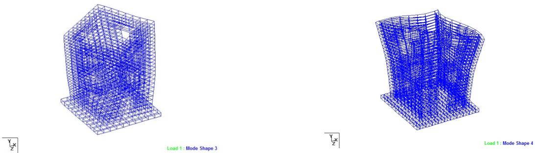
1<sup>st</sup> Torsion mode shape in Model 3 (Mode 3, 4.021 Hz)      1<sup>st</sup> Torsion mode shape in Model 4 (Mode 4, 7.11 Hz)
