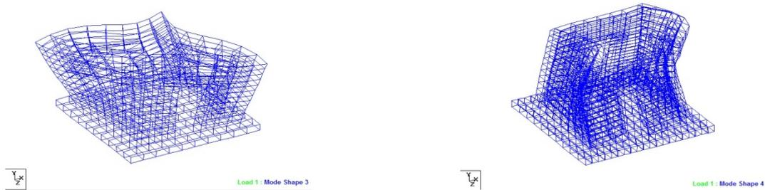
1<sup>st</sup> Torsion mode shape in Model 1 (Mode 3, 6.293 Hz)      1<sup>st</sup> Torsion mode shape in Model 2 (Mode 4, 9.166 Hz)
