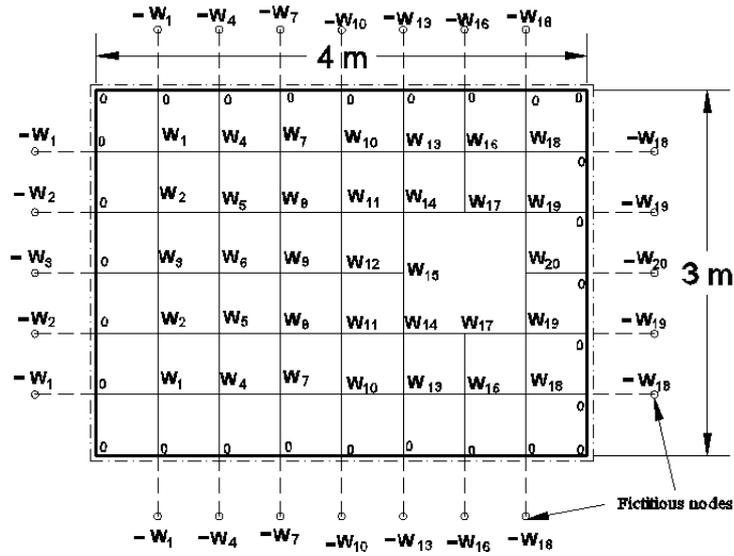
Figure 3. Experimental plate with unknown node displacement
