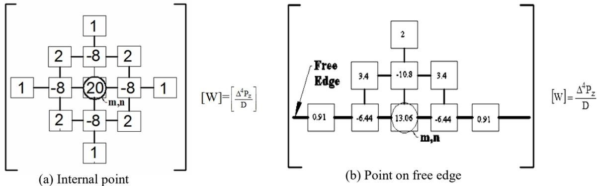
Figure 2. Graphical presentation of FDM expressions for different node location.
