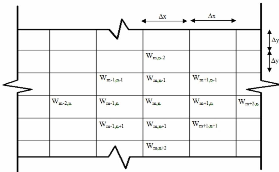
Figure 1. Plate element with nodes and deflection components
