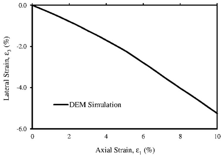
Figure 2. Relationship between the axial strain,  $\epsilon_1$  and lateral strain,  $\epsilon_3$  during the simulation
