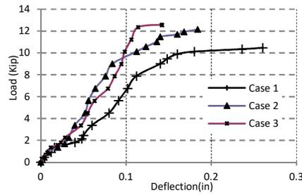
Figure 3. Load-deflection curves of experimental beams
