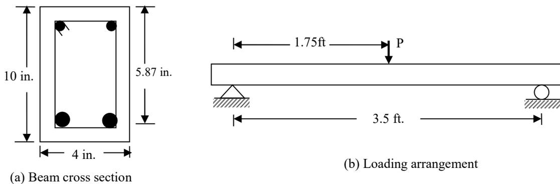
Figure 1. Beam cross section and loading arrangement
