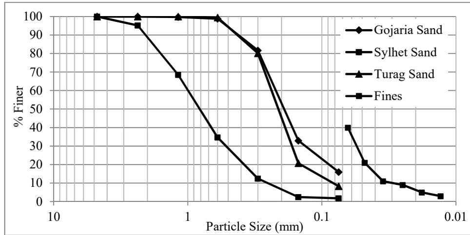
Figure 1. Grain size distribution curves of collected soil samples and fines
