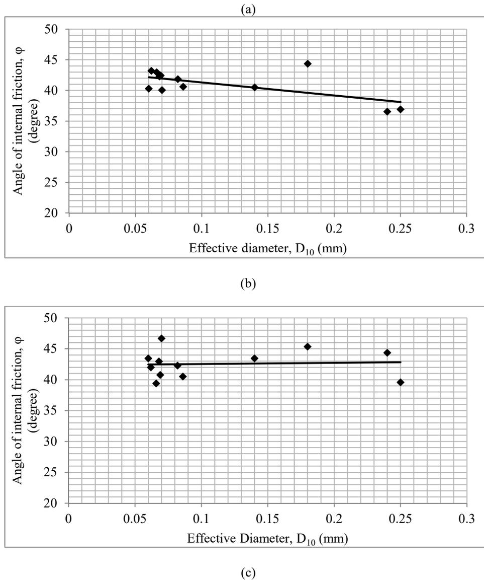
Figure 2. Variation of frictional angle with effective size at density (a) 15.2 kN/m<sup>3</sup>(b) 15.8 kN/m<sup>3</sup>(c) 16.5 kN/m<sup>3</sup>
