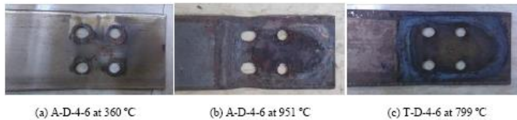
Figure 6. Failure mode of two-parallel bolted connection specimens at elevated temperatures
