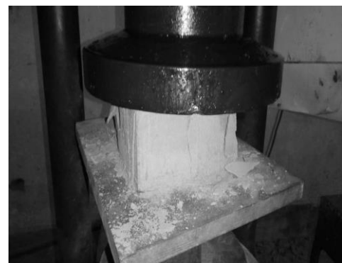
Figure 7. Fly Ash brick in compression
