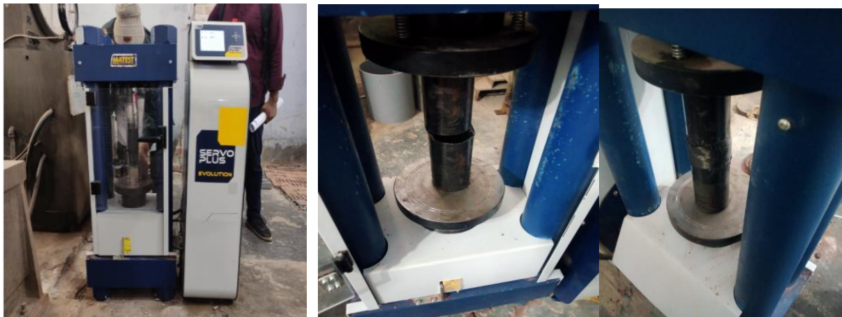
Figure 8. Test Setup and failure mode of deficient CFRP strengthening short column
