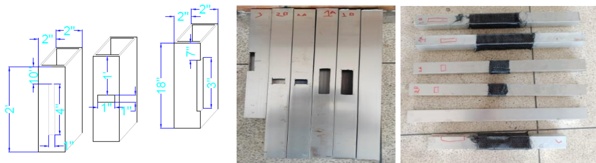
Figure 3. Dimensions, deficient and CFRP strengthen test aluminum specimen
