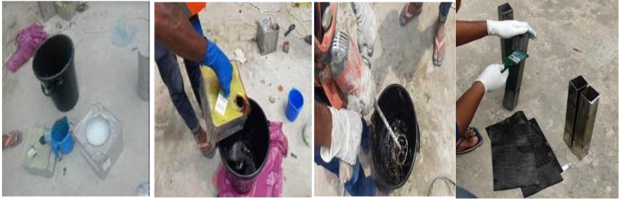
Figure 6. Mixing primer and base resin & hardener adhesive
