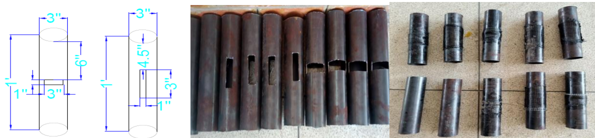
Figure 5. Dimensions, deficient and CFRP strengthen test mild steel specimen
