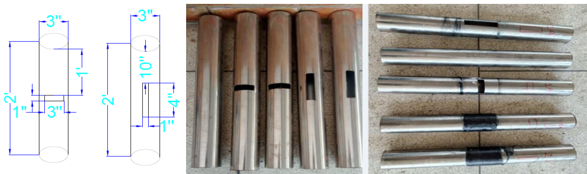
Figure 4. Dimensions, deficient and CFRP strengthen test stainless steel specimen
