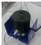
Figure 5: The modal shaker (TMS 2100E11).
