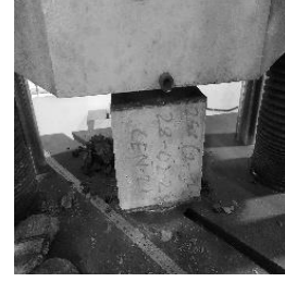
Figure 7. specimen testing by UTM
