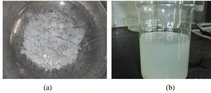
Figure 5. (a) Sodium Hydroxide Pellets and (b) Sodium Silicate Solution
