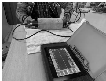
Figure 4: Testing specimen using UPV
