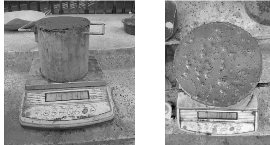
Figure 2: Weighting container with fresh concrete
