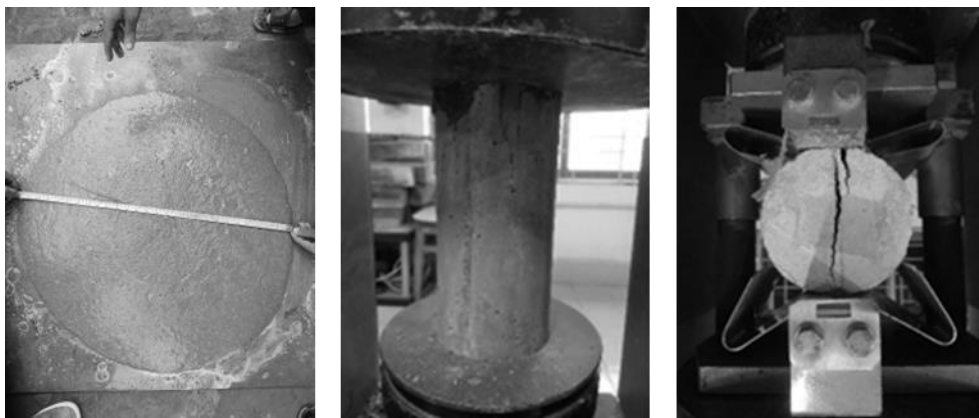
Figure 2. Slump flow, compressive and splitting tensile strength test arrangements.
