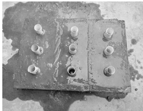
Figure 5. Casting of the mortar
