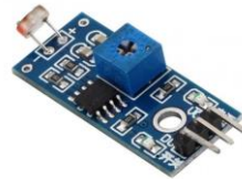
Figure 6. LDR Sensor Module
