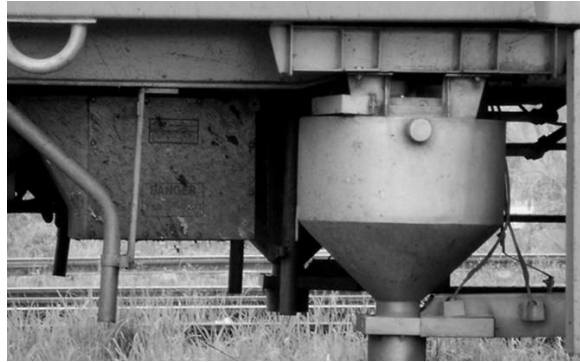
Figure 5. Controlled Discharge Toilet System (CDTS) Tank Beneath the Coach
