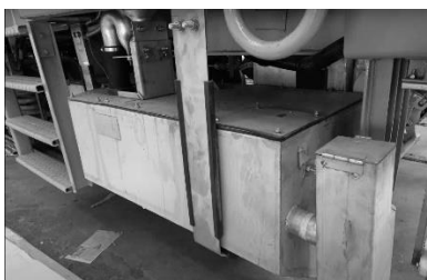
Figure 6. Position of Bio-digester Tank (DRDO & IR, 2015)
