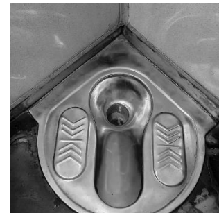
Figure 3. Traditional Hole in Floor Toilet in LHB Coaches (Indian Rail Info, 2022)
