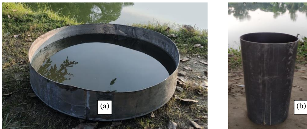
Figure 1: Water loss measurement instruments: (a) USWB Class A Evaporation Pan, (b) Single Ring Infiltrimeter
