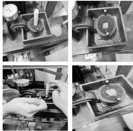
Figure 3. Direct shear test set up
