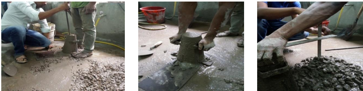
Figure 2. Trial Mix Slump test being performed
