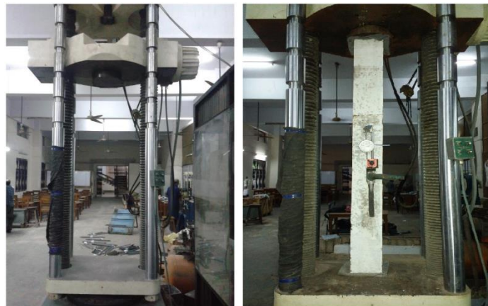
Figure 4. TINIUS OLSEN MACHINE and RC column set up
