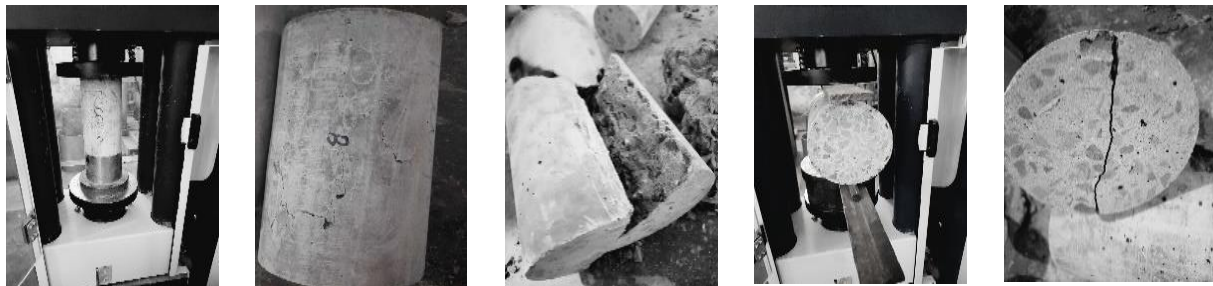
Figure 6. Compressive Strength and Splitting Tensile Strength Testing.
