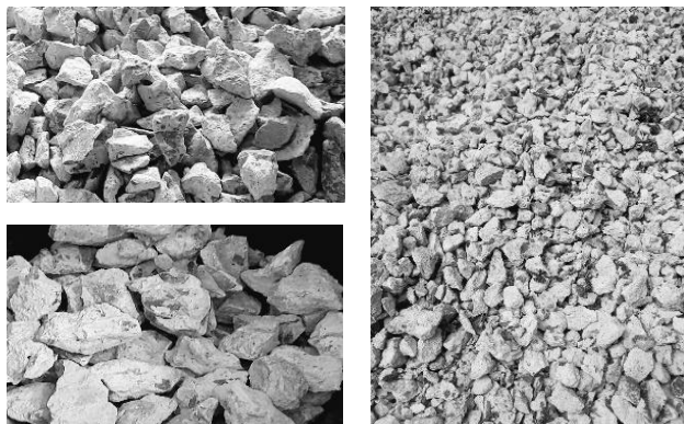
Figure 1. RCA from demolished pile head.
