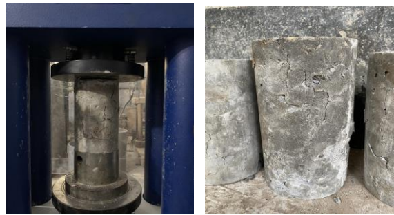
Figure 4. Compressive strength test of specimens
