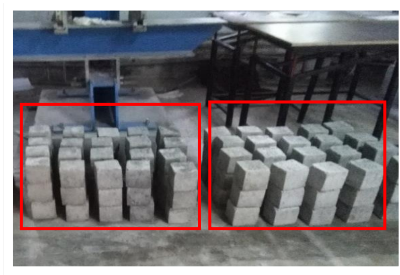
Figure 1. From Left (a) specimens exposed to sodium chloride environment and (b) Specimen exposed to plain water
