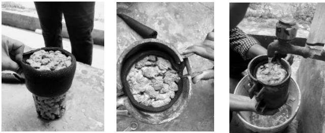
Figure 4: Permeability test of PC
