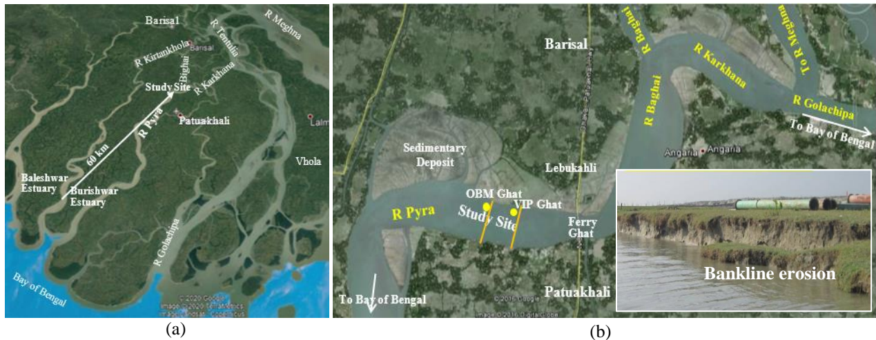
Figure 1: (a) Overall study area with surrounding districts, river system and estuary, (b) Study site details, 22.274490°N, 90.173525°E to 22.301957°N, 90.214919°E. ADCP run lines ( — ), sediment sample, water level data location ( ● ), Inset: Bank line erosion scenario
